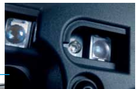
Beissbarth reference system with 2 cameras per sensor
