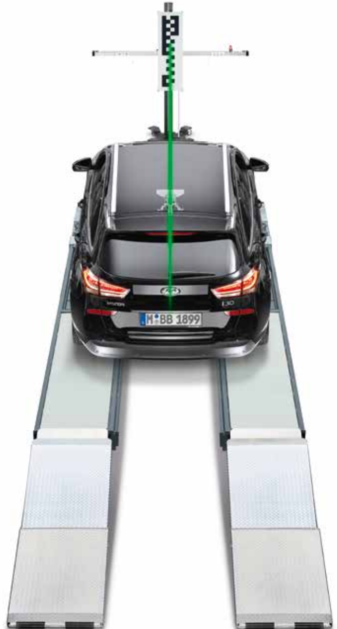
Hyundai with BBFAS 415 Universal calibration target type 1S
