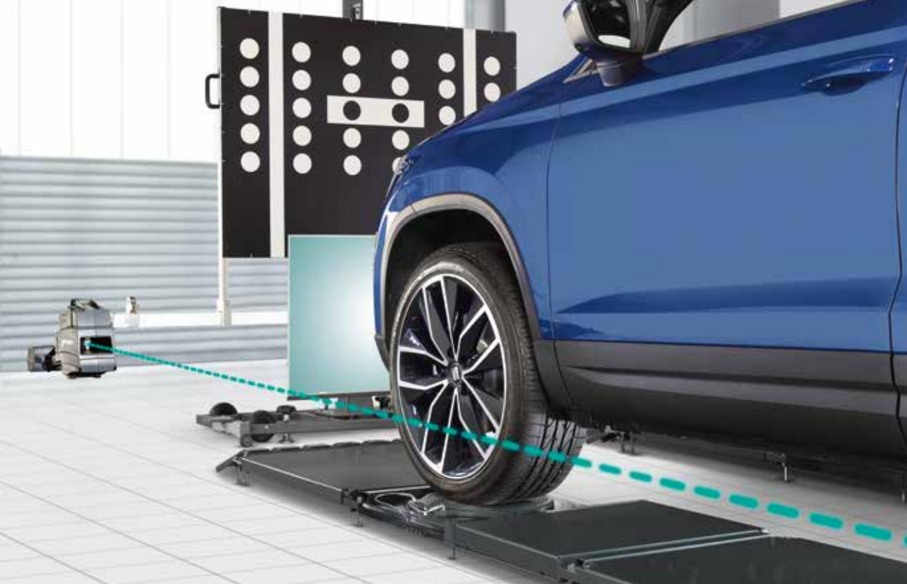
DAS adjustment using Easy CCD+
