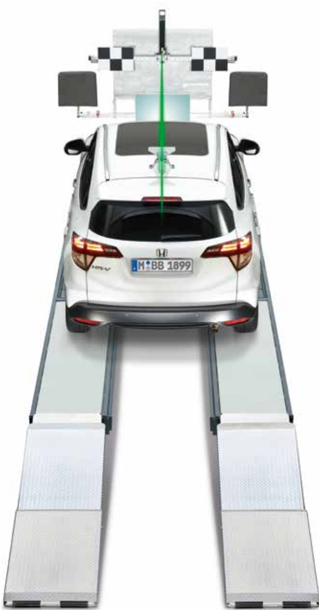
Honda HRV with BBFAS 1000 with BBFAS 1415 retrofitting kit Honda calibration target type 1
